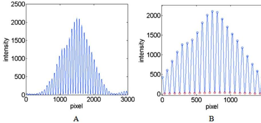
FIG. 1. (Color online) (A) Smoothed interference pattern. The slight asymmetry in the interference pattern was due to minor misalignments in the optical apparatus. (B) Center segment, with minima and maxima identified. The y-axis is the level of illumination intensity returned by the Thorlabs camera.
