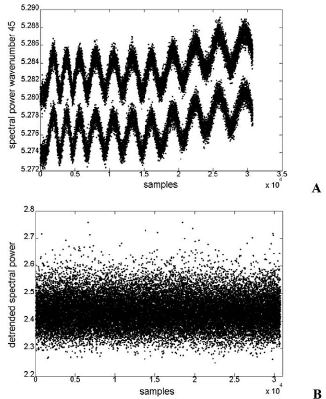
FIG. 2. (A) Double-slit spectral magnitude at wavenumber 45 across 30,000 camera frames (one sample per frame), showing bimodal distribution. (B) Same after linear detrending the spectral magnitude between single and double-slit peaks (from wavenumbers 14 to 39).
