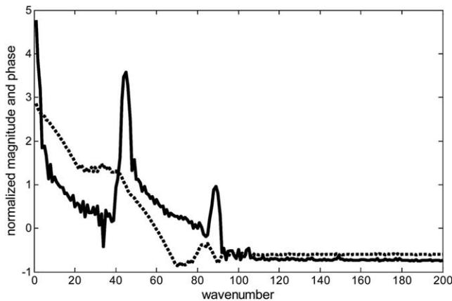
FIG. 1. Mean normalized log 10 spectral magnitude (solid line) and mean normalized unwrapped phase (dotted line) for wavenumbers 1–200, averaged across a sample dataset of 30,000 interference patterns. The magnitude peak at wavenumber 2 corresponds to the diffraction pattern associated with each slit; the peak at wavenumber 45 corresponds to the interference pattern created by both slits; the smaller peak at wavenumber 90 is a harmonic of the peak at 45.
