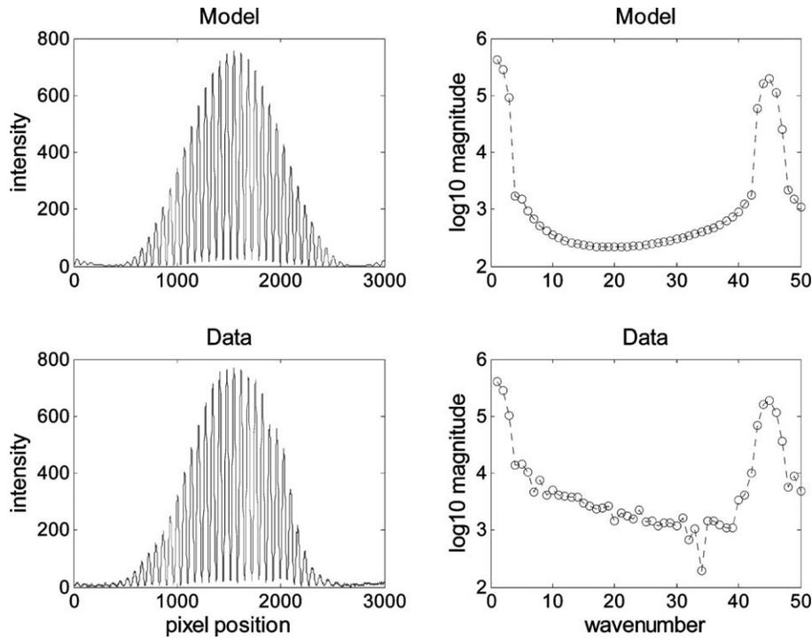
FIG. 7. Comparison of observed and modeled interference patterns and associated log spectral magnitude for first 50 wavenumbers. Note that the modeled value at wavenumber 45, which corresponds to the spectral power of the double-slit interference pattern, closely matches the value observed in the actual data.
