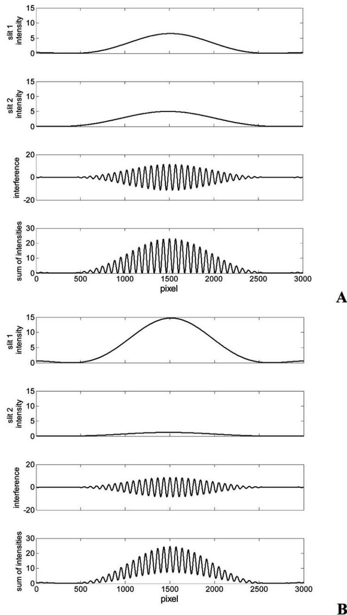
FIG. 9. (A) Illumination intensity resulting from each slit, interference between the slits, and the modeled interference pattern, when the electric field ratio  $A/B = 1$ . (B) The same measures when this ratio is unbalanced at  $A/B = 3$ .
