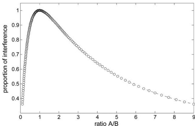
FIG. 8. Relationship between the ratio of electric field intensity passing through slit 1 versus slit 2,  $A/B$ , and the proportion of resulting interference (i.e., 1 is maximal interference, 0.5 is half the maximum interference).
