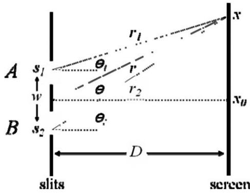
FIG. 6. Parameters associated with a Fraunhofer model of a double-slit optical system. Parameters  $A$  and  $B$  are electric field strengths associated with the light beam passing through slits 1 and 2, respectively. See text for description of the other parameters.
