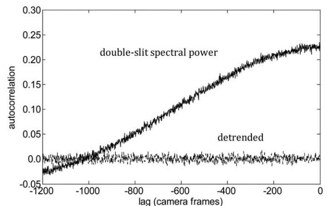
FIG. 3. Autocorrelations up to lag 1200 in successive samples of double-slit magnitude (i.e., wavenumber 45) and autocorrelations after linearly detrending.
